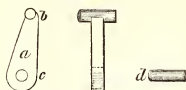
Fig. 20. Mainspring-swivel , full size. a , body; b , axis; c , tumbler-pin hole; d , tumbler-pin.
