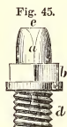
Fig. 45. Cone, full size, (spare.) a, nipple; b, square; c, shoulder; d, screw-thread; e, vent.
